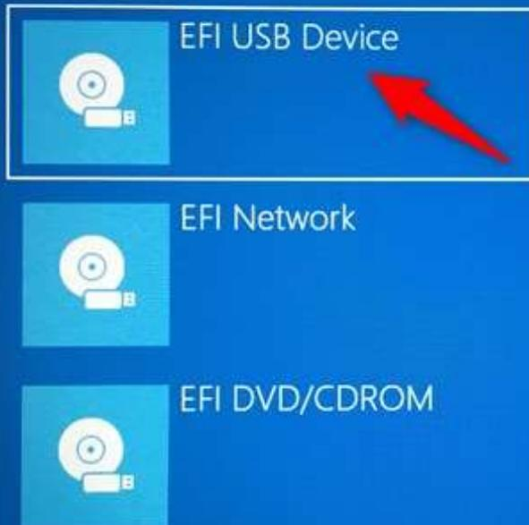
Selecting the USB flash drive from which the PC should boot
